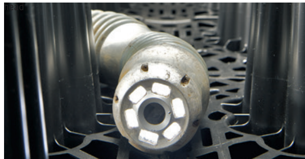
Push camera, cleaning equipment with a rinsing
